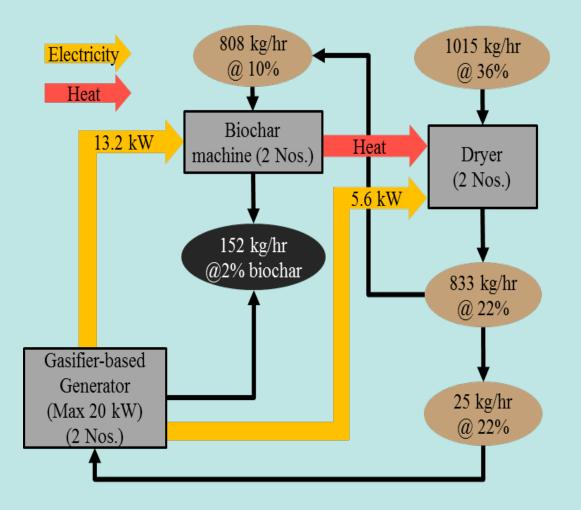
Mass balance, heat, and electricity requirements of an integrated biochar production system
